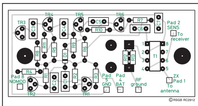
Fig 4: The component layout on the PCB.
